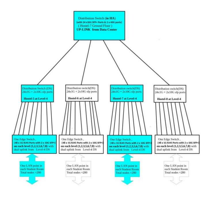
Fig: Network Diagram for Hostel LAN Connectivity
