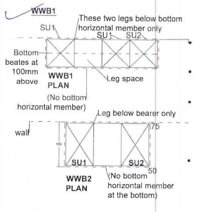
Granite top projection 75mm at the back(No rounding)with 100 high splashrack of same material Other 3 sides projected to be 50mm top edge \( \frac{1}{4} \) rounded and polished Note; where 2 unit are fomed that side not to be rounded but straight cut and polished
