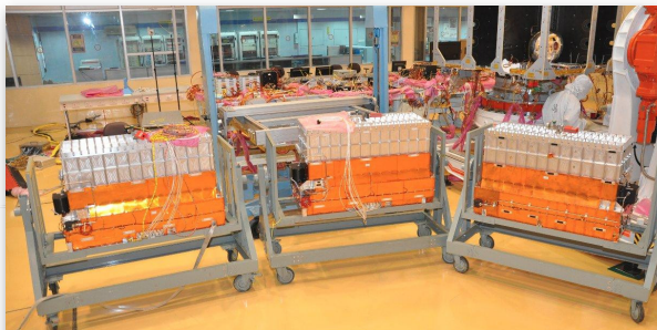
The LAXPC Detectors in clean room during integration on AstroSat.
