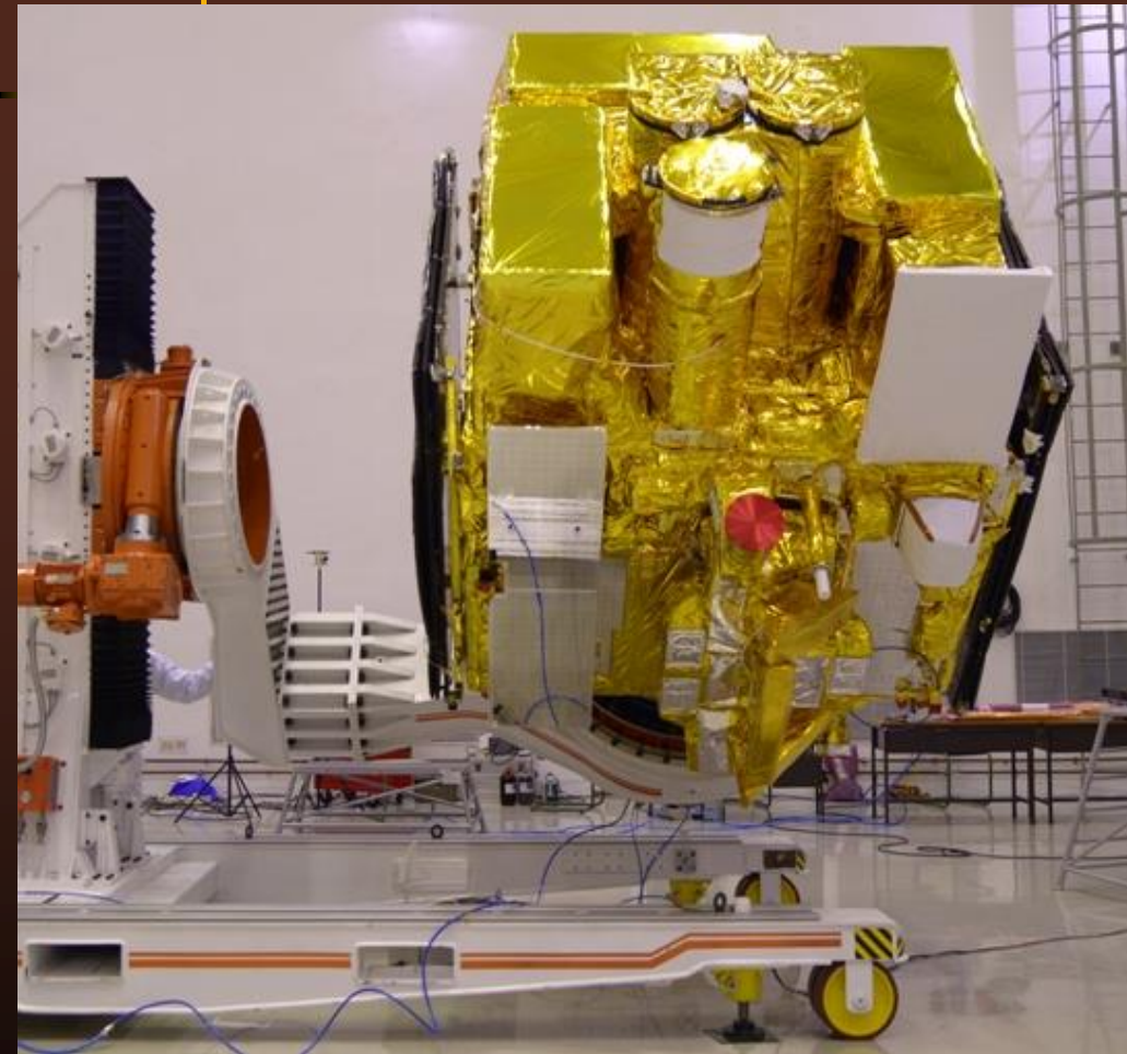
S/C in tilted position during pre-launch test at SHAR
