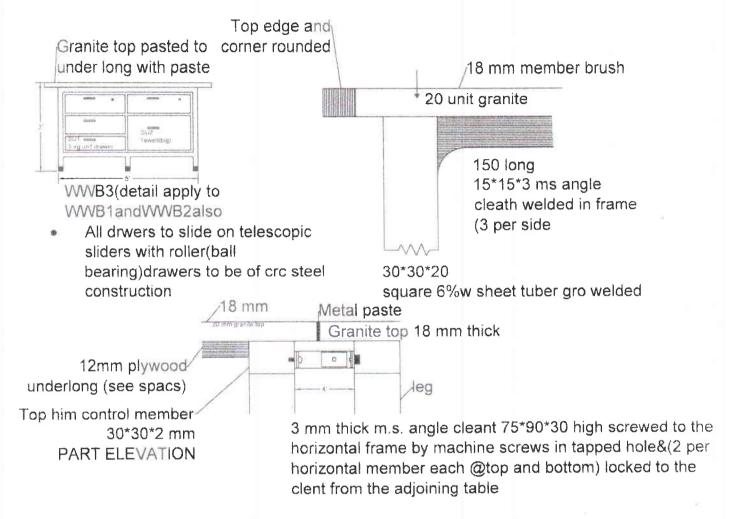
T Tpical detail for connecting work benches (after installation)
