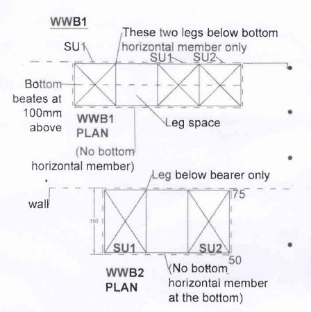
Granite top projection 75mm at the back(No rounding)with 100 high splashrack of same material Other 3 sides projected to be 50mm top edge \( \frac{1}{4} \) rounded and polished Note; where 2 unit are fomed that side not to be rounded but straight cut and polished
