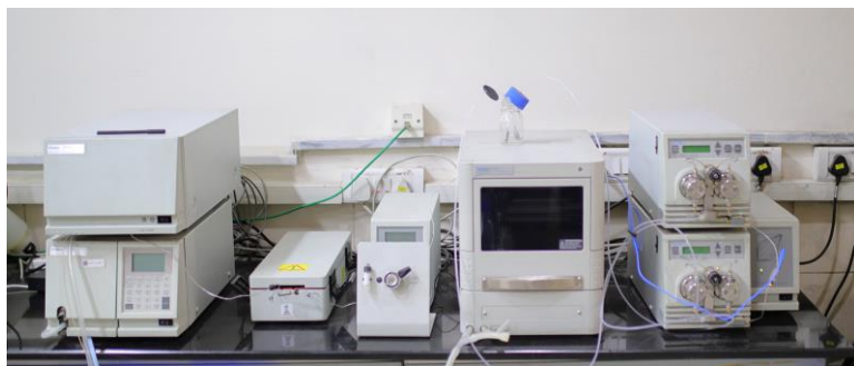
High-Performance Liquid Chromatography with 2707 Autosampler and 2998 Photo Diode Array detector
